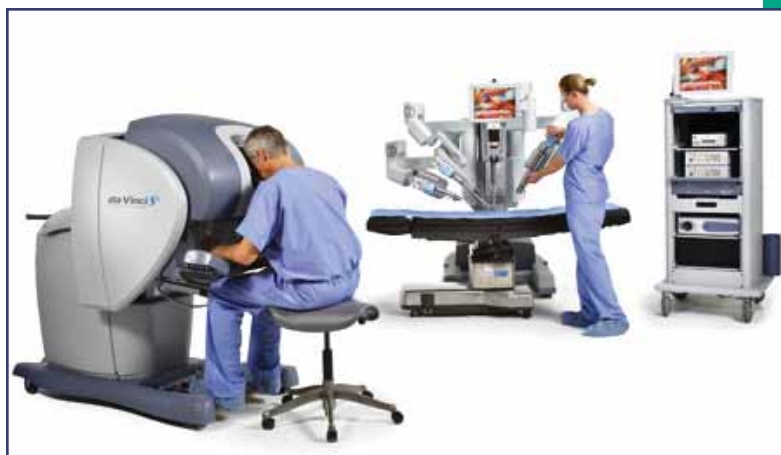
A surgeon sits at the console, while a nurse shows the robotic arms
